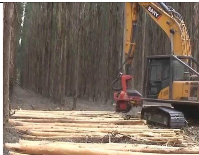
On-site Harvester cum De- Barking Machine
