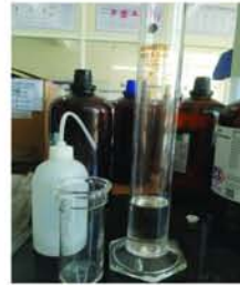
150ml solvent added into the extraction beaker and transferred into extraction beaker
