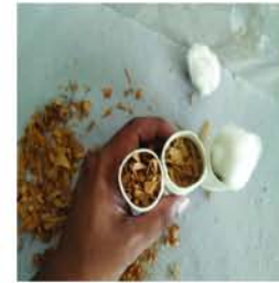
Transferred into cellulose thimble covered with cotton plug
